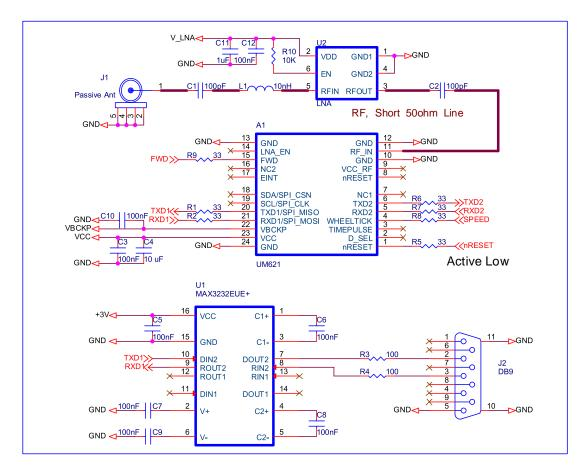
Figure 2-1 Reference Circuit Using a Passive Antenna
