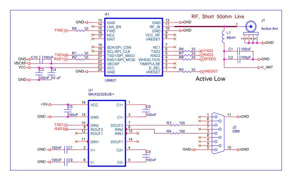
Figure 1-1 Reference Circuit Using an Active Antenna
